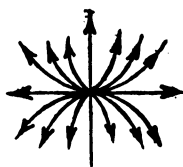
Fig. 2. Roots \lambda real and both > 0 . Instability.
